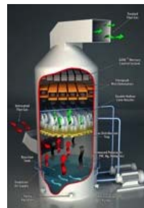
排煙脱硫 (FGD) (SO 2 )
